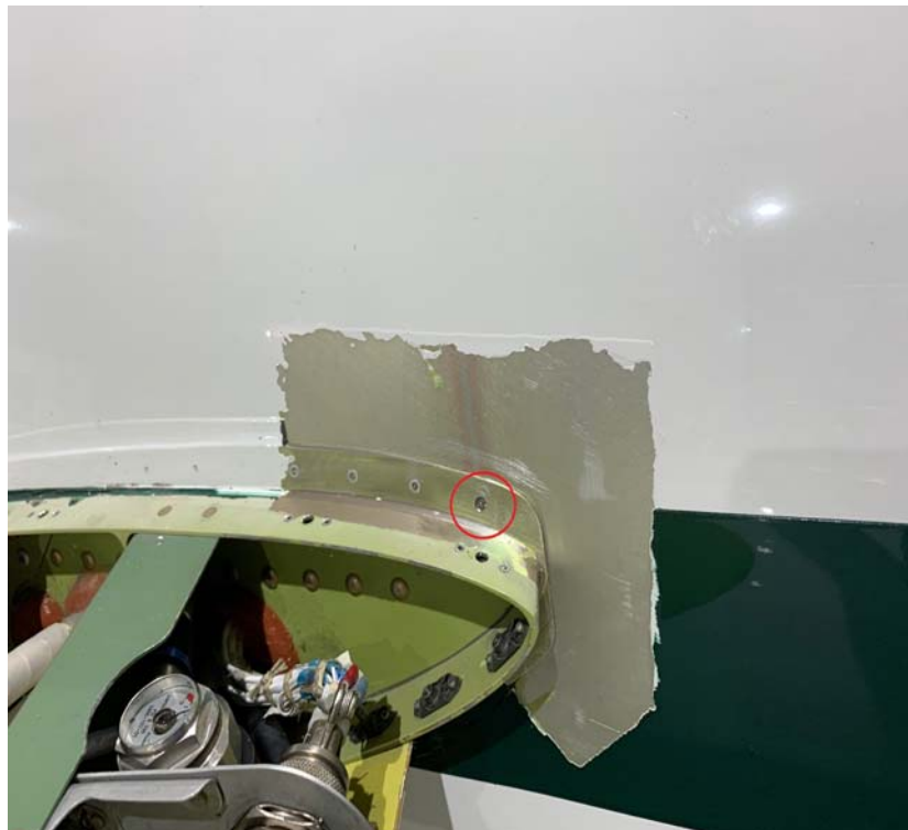
Figure 3. Example of Damage - Paint Removed
